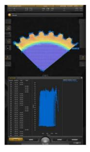
Optional Color Hardness Contour Map displays sample hardness and location with a color representation of hardness variances.
