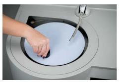
Manually polish samples safely and efficiently.
